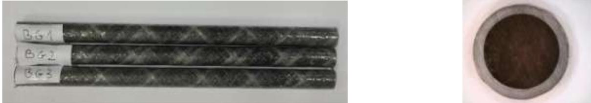
**Fig. 3:** Hybrid bars manufactured by the pultrusion and filament winding method. The structure consists of CFRP core and GFRP filament-wound overwrap
