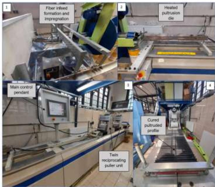
**Fig. 1:** Pultrusion system. 1 - Resin impregnating unit, 2 - curing unit, 3 - pulling and control unit, 4 - cutting unit
