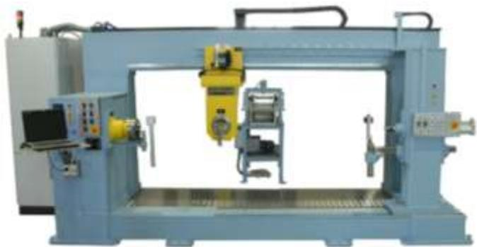
**Fig. 2:** Machine for the filament winding method
