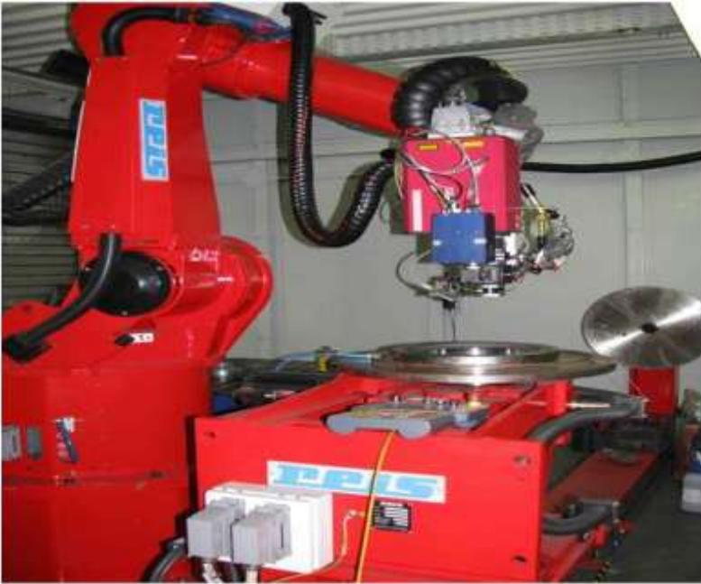
Fig. 1: Robot laser cell for hardening
