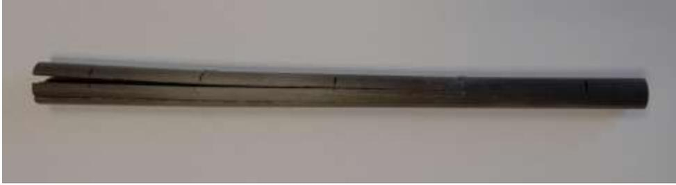
**Fig. 7:** Smooth CFRP bar after bending test. These samples show the brittle nature of such a structure with the type of delamination damage.
