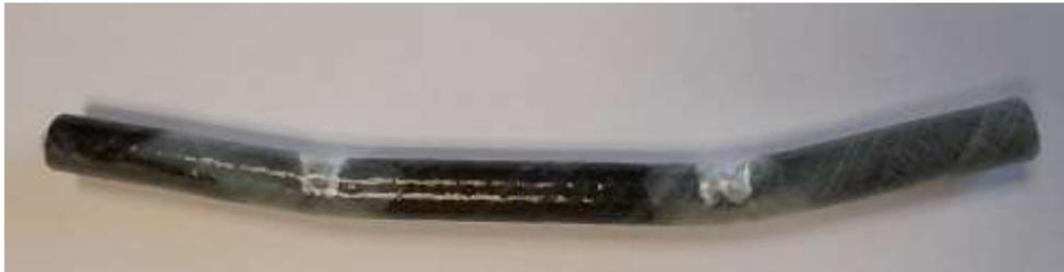
**Fig. 5:** Hybrid bar after bending test. Visible local failures at the places of the applied force (load support). The white areas around suggest cracking of the matrix.
