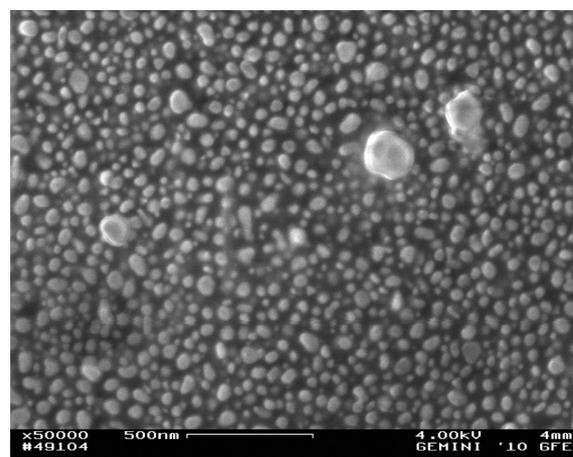
Figure 7: SEM image of Au nanoparticles (synthesis parameters: 260 °C, 2.5 MHz)
