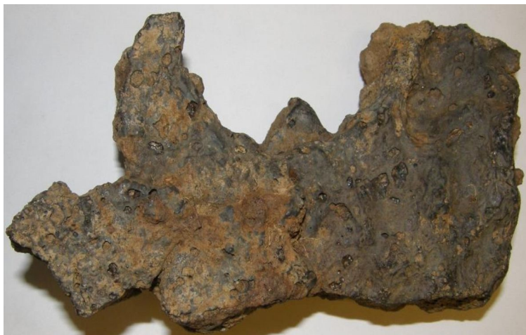
Fig. 9: Piece from the shaft at the site Vårhussetra, with the half of an opening measuring 8 cm. Thickness 20-25 mm. In spite of careful studies of the slag ps this is the only representing an air inlet. The diameter tells that air was admitted without using bellows, which seem to have nossels not exceeding 1 inch. On the back side there is grey clay. The piece has a slight curvature like the other pieces of the shaft. It can for good reason be regarded as a part of the wall. (Photo Arne Espelund)
