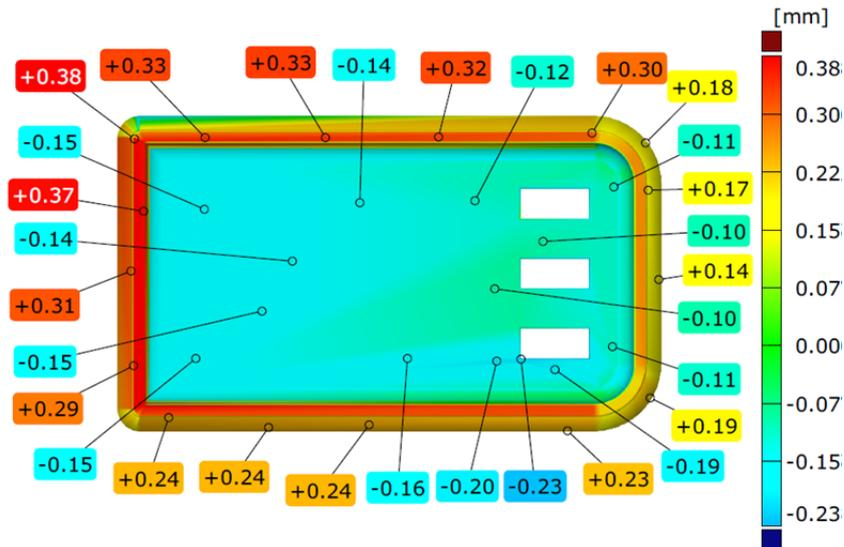
Fig. 12 Deviations of back camera cover – rear view
