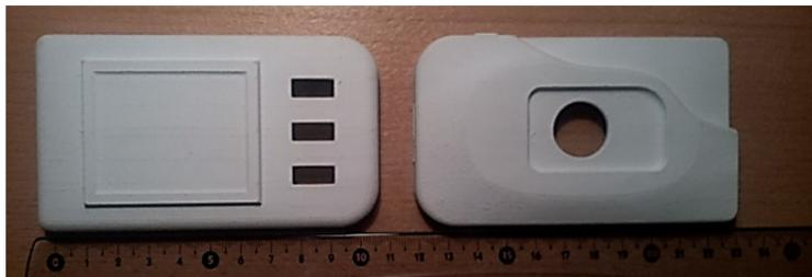
**Fig. 2** 3D printed models of camera casing
