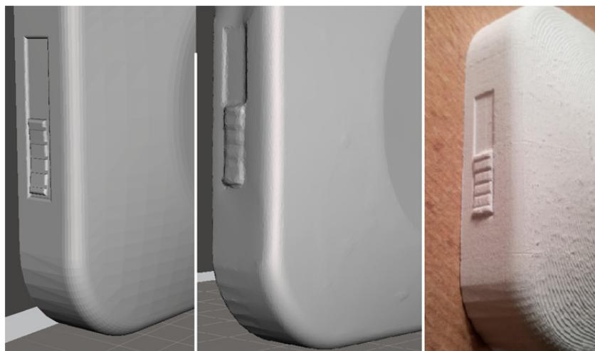
**Fig. 5** Detail of original (left), scanned (middle) and printed (right) front camera cover
