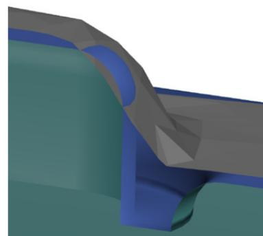
Fig. 14 Generated model (blue) and scanned model (grey)
