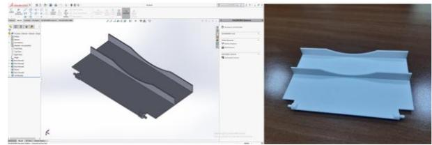
Figure 11. Drawing of the shutter on the pool and a prototype of the shutter made by 3D printing
