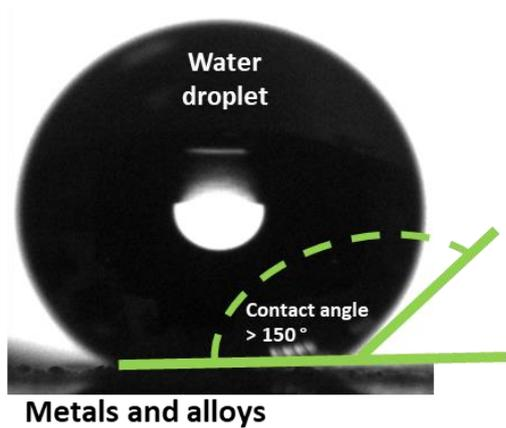
*Figure 1: Water droplet on the superhydrophobic surface with contact angle above 150°*
