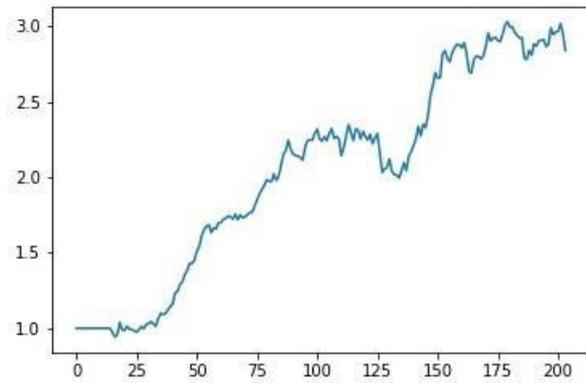
Figure 2: Estimated cutting tool wear during cycles until the cutting tool replacement. Anže Marinko. 2021.
