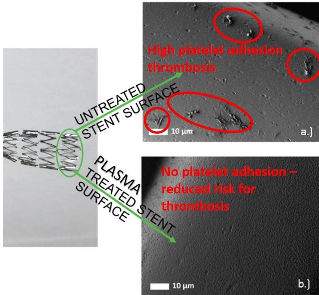
Figure 1: On the left-hand side bare metal vascular stent from NiTi alloy (Kindly donated by Rontis AG) is shown, while stent surface after incubation with whole blood is presented on the right-hand side. Interaction of platelets with the surface of commercial and plasma-treated vascular stent (images obtained from scanning electron microscopy) is shown. Ita Junkar. 2021.
