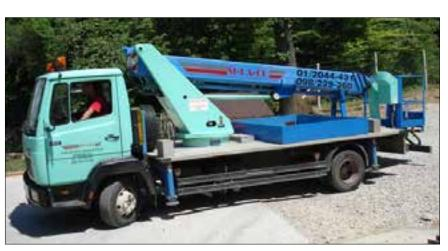
Figure 1. Mobile hydraulic platform Wumag WT 225
