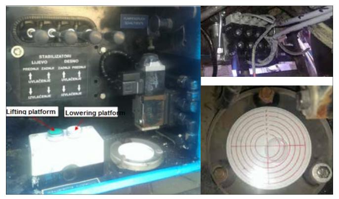
**Figure 3.** Cabinet for automatic levelling after reconstruction procedure, hidraulic distributors for nivelation process and circular libelle
