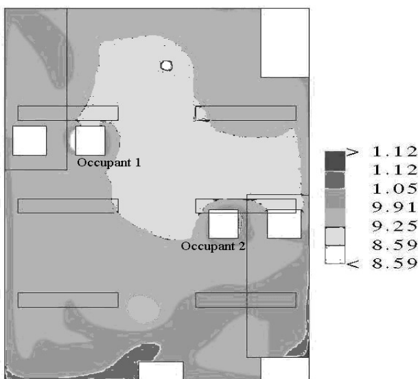
Sl. 3. Sobna koncentracija radona v \text{Bq/m}^3 pri 0,5 stopnji izmenjavanja zraka in višini 1,2 m (prerez X-X') Fig. 3. Room radon concentration in \text{Bq/m}^3 at 0.5 air-exchange rate and 1.2 m height (Section X-X')
