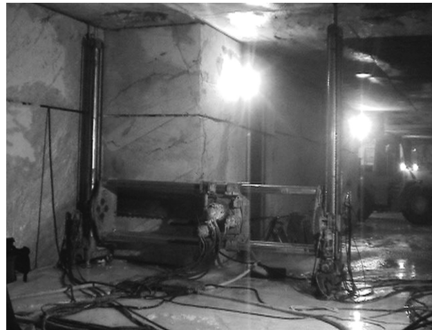
Figure 1: Column-driven chainsaw machine Fantini G.70 on the location in the Hotavlje I quarry
