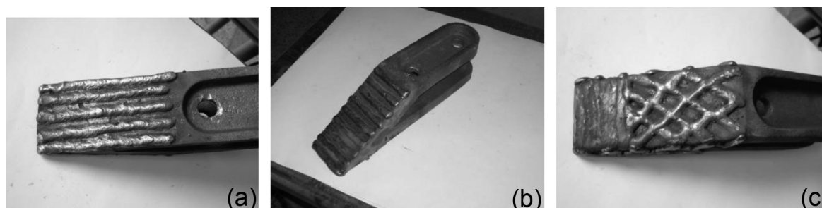
Figure 9: Hardfaced teeth with the layers deposited: a) longitudinally, b) horizontally and c) in a honeycomb pattern
