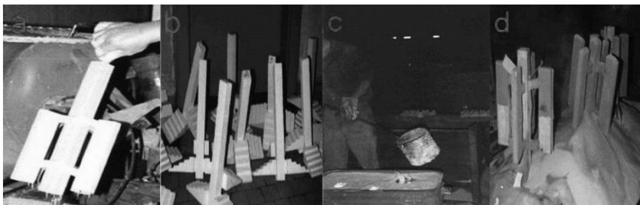
Figure 2: Lost-foam-process phases: a) coating-excess removal from the pattern and layer equalizing on the pattern surface, b) coating-layer drying, c) staged probe prepared for casting, d) easy coating removal from the casts
