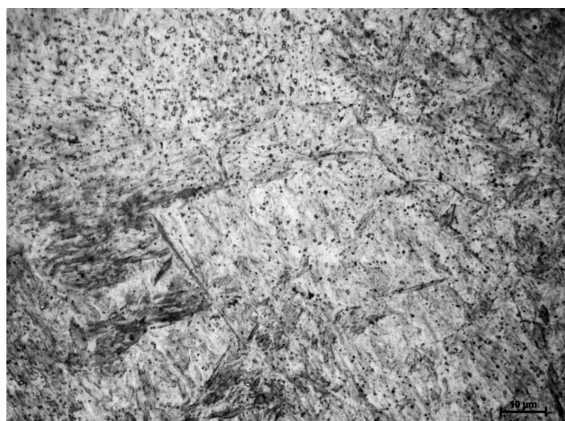
Figure 10: Microstructure of 2T specimen; etched in Vilella-Bain
