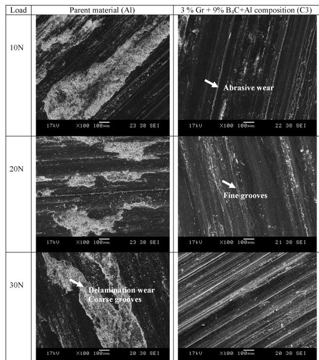
Figure 5: SEM micrographs of the worn surfaces of hybrid Al-B<sub>4</sub>C composites and aluminum (sliding speed 1 m/s, sliding distance 2500 m)
