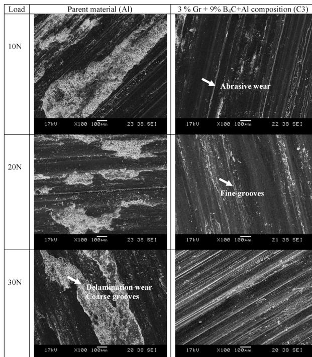
**Figure 6:** SEM micrographs of the worn surfaces of hybrid Al-B<sub>4</sub>C composites and aluminum (sliding speed 2 m/s, sliding distance 2500 m)
