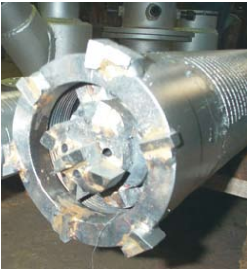
Figure 6. Filter with \phi 128 mm diameter, a drilling crown with cutting diameter of \phi 148 mm, fixed to the screen, and removable crown Slika 6. Filter premera \phi 128 mm, vrtna krona z rezalnim premerom \phi 148 mm, ki je fiksirana na filtru in izvlačljiva krona
