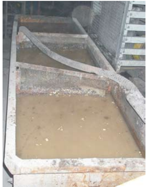
Figure 5. Preparation of the drilling fluid Slika 5. Priprava izplake
