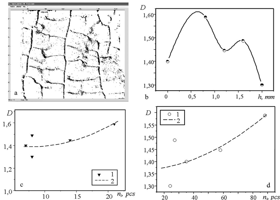
Figure 1: Analysis of the multiple cracking surface: a) image of surface; b) change a fractal dimension on the depth of analyzable area; c) dependence of fractal dimension on the quantity of identified coalesced cracks and d) individual cracks; 1 – experimental data; 2 – approximation
