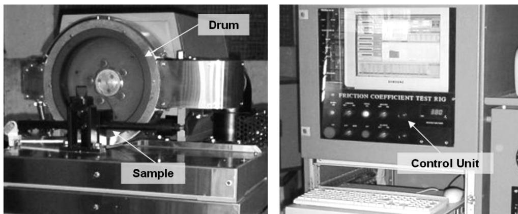
**Figure 1:** Chase-type friction tester
