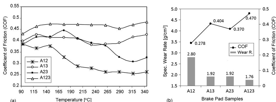
**Figure 4:** Friction-test results for A12, A13, A23 and A123 brake-pad materials: a) *COF* depending on the test temperature (°C), b) the average *COF* at elevated temperatures and specific wear rates
