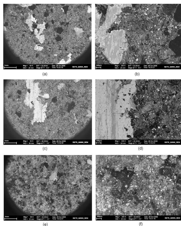
**Figure 3:** SEM micrographs of the worn surfaces of the brake-pad specimens after the friction test: a) A1-general, b) A1-detailed, c) A2-general, d) A2-detailed, e) A3-general and f) A3-detailed
