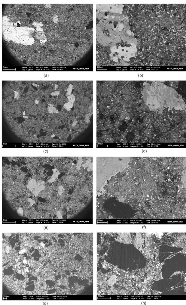
**Figure 5:** SEM micrographs of the worn surfaces of the composites in the Chase test machine: a) A12-general, b) A12-detailed, c) A13-general, d) A13-detailed, e) A23-general, f) A23-detailed, g) A123-general, h) A123-detailed
