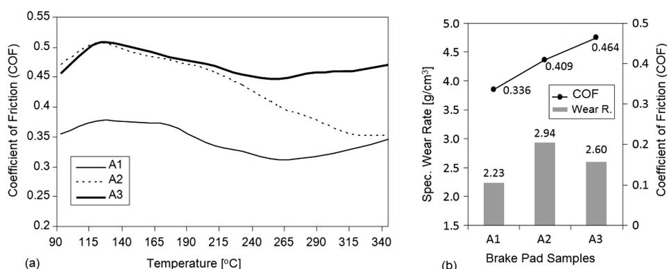
**Figure 2:** Friction test results for A1, A2 and A3 brake-pad materials: a) *COF* depending on the test temperature (°C), b) the average *COF* at elevated temperatures and specific-wear rates
