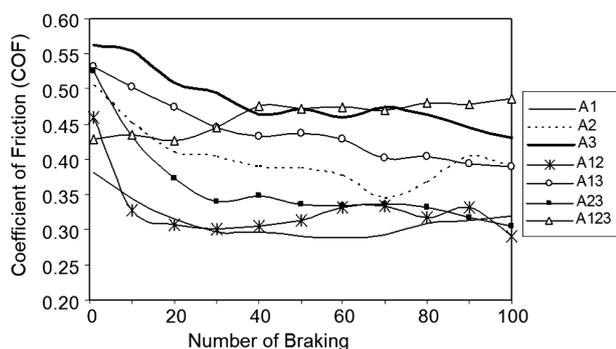
**Figure 6:** *COF* variations related to the number of brakings for the A1, A2, A3, A12, A13, A23, A123 brake-pad materials
