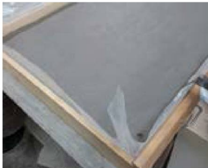
Slika 1: Plošča OPMIS-2 (še v kalupu – vidna zgornja stran) Figure 1: Hydraulically bound fiberboard OPMIS-2 (in mold – upper side is visible)
