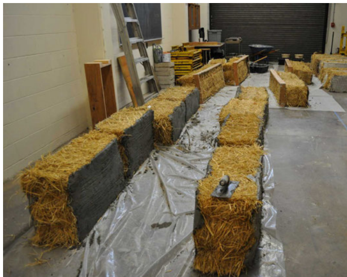
Slika 3: Priprava merjencev – nanos ometa na bale slame. Figure 3: Specimen preparation – straw bale plastering.
