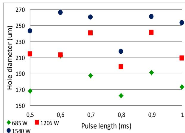
**Fig. 6** The entrance diameter of the holes drilled in alumina ceramics by QCW fiber laser in dependence on pulse length for three peak powers by keeping frequency 50 Hz and number of pulses 100
