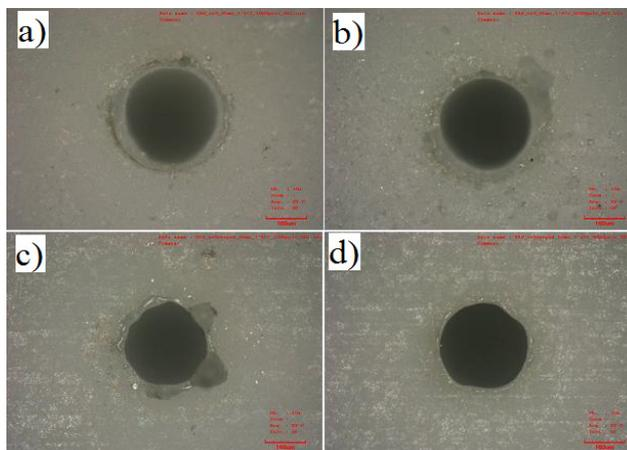
**Fig. 2** Images of holes in alumina ceramics drilled by Nd:YAG laser obtained at process parameters of pulse length 0.5 ms, frequency 20 Hz and pulse energy 1.47 J: a) entrance, 20 pulses, b) entrance, 160 pulses, c) exit, 20 pulses, d) exit, 160 pulses. Magnification 240x, red scale 160 µm.
