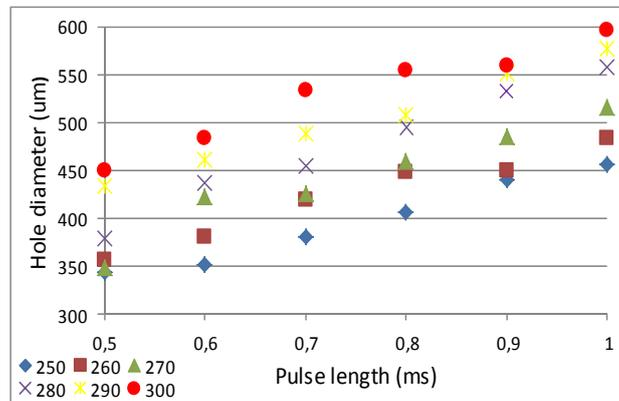
**Fig. 3** The entrance diameter of the holes drilled in alumina ceramics by Nd:YAG laser in dependence on pulse length for six charging voltages in the range from 250 V to 300 V by keeping frequency 20 Hz
