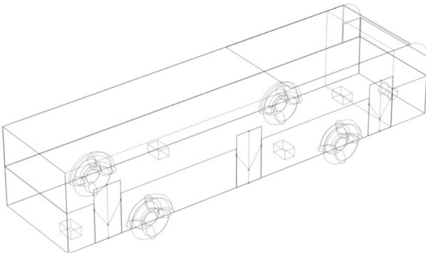
**Figure 2:** Heater positions inside the electric bus
