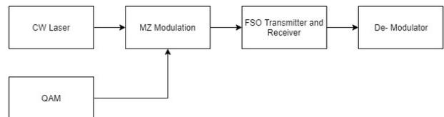
**Figure 9.** Radio over Free Space Optics where modulated signals are transmitted over free air.
