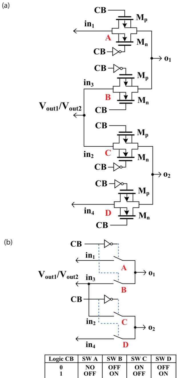
**Figure 8:** Analog switch implementation: (a) circuit, (b) symbol.
