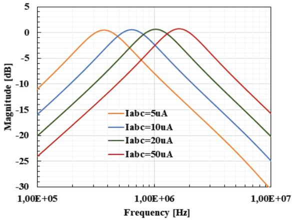
**Figure 11:** Simulated frequency responses of BP with different  $\omega_0$ .
