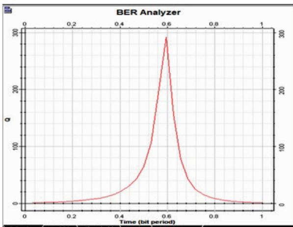
Figure 14: Q-factor of DCF over bit period
