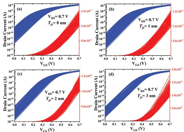
**Figure 3:** (a)–(d) ID-VG transfer characteristics of NCJL-FinFET with different thicknesses of ferroelectric layers
