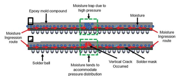
**Figure 6:** Schematic illustration to describe crack phenomena, (A) moisture ingress route and trap at the middle, (B) moisture tend to find possible route to accommodate pressure distribution
