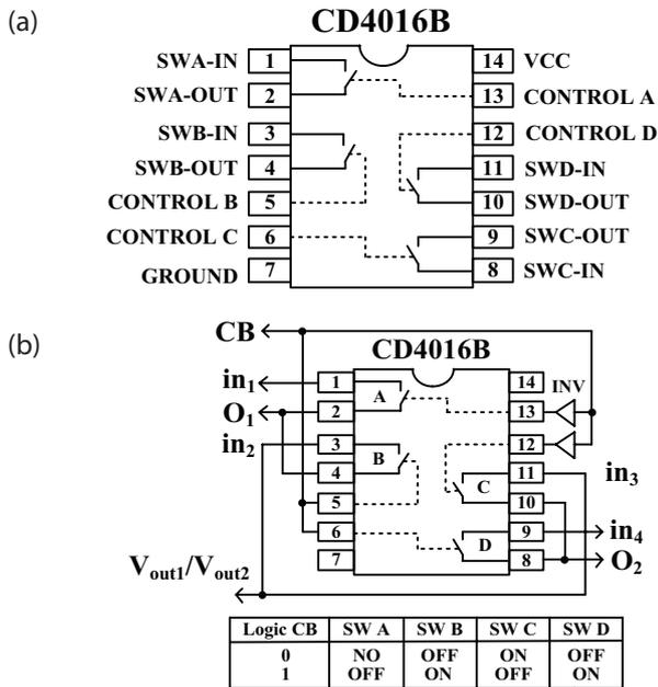
**Figure 20:** 4-channel analog switch CD4016B: (a) CD4016B pinout, (b) Implementation for SW<sub>1</sub> and SW<sub>2</sub>.
