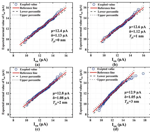
**Figure 5:** (a)–(d) Expected normal value of the ON-state current ( $I_{on}$ ) and simulated value of the actual device model
