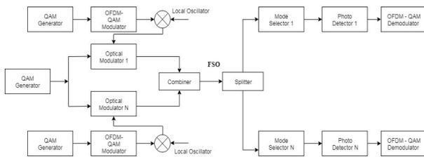
**Figure 10:** High-Capacity Ro-FSO Transmission with Mode Division Multiplexing.
