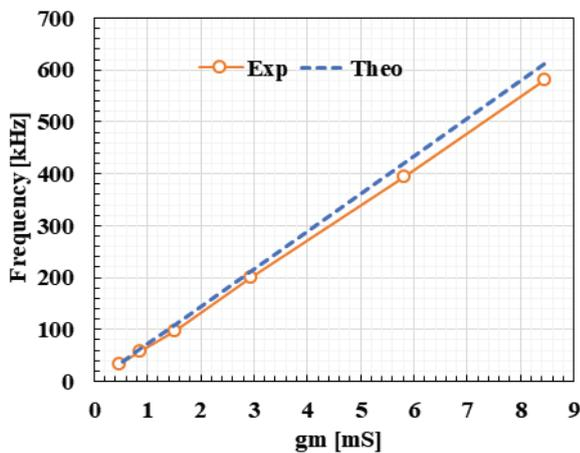
Figure 29: The frequency of oscillation against transconductances  $g_m$ .
