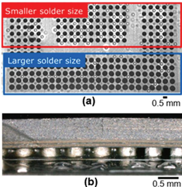
**Figure 2:** Micrograph of: (a) different size and location of solder ball from X-ray testing after reflow soldering process and (b) side view image of solder ball at the middle showing slightly elongated than that of the edge location
