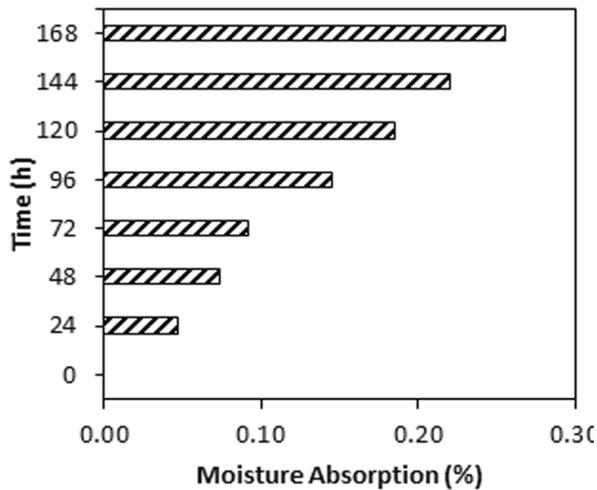
**Figure 1:** The moisture absorption of the samples at conditioning setting of 30°C/60%RH/168 h
