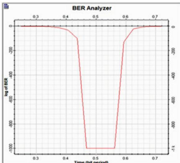
**Figure 12:** BER curve of FBG over bit period
