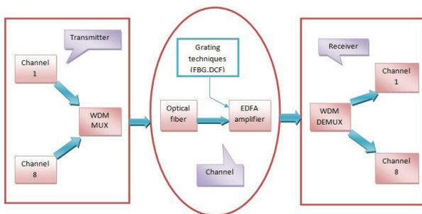
**Figure 1:** Block diagram of WDM MIMO 8 x 1 channel with Compensation techniques using (FBG and DCF).
