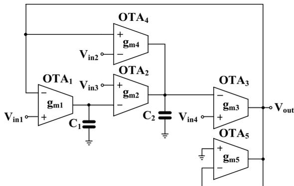
**Figure 2:** Universal biquad filter using single output OTAs.
