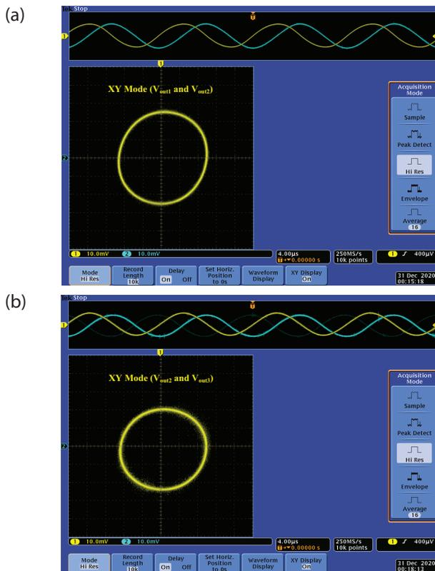
Figure 28: Lissajous pattern: (a)  $V_{out1}$  and  $V_{out2}$  outputs, (b)  $V_{out2}$  and  $V_{out3}$  outputs.
