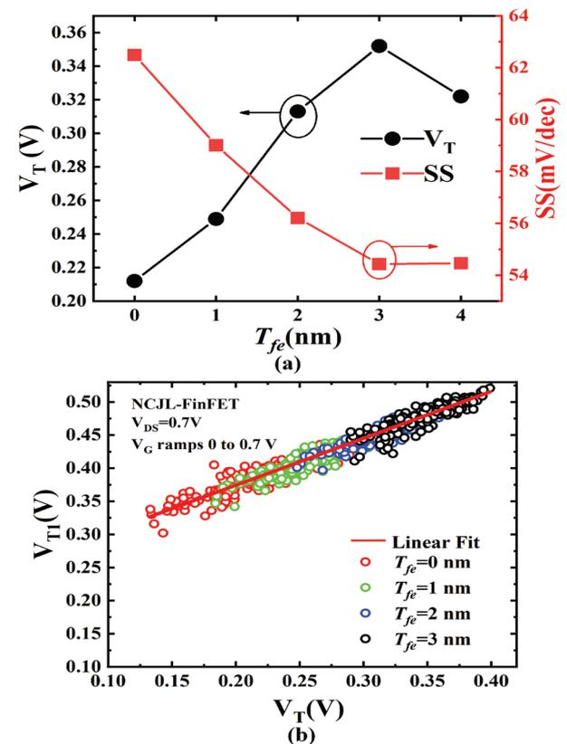
**Figure 4:** (a) Variation of threshold voltage with the thickness of ferroelectric layer and (b) The shift trend and dispersion between  $V_T$  (is extracted gate voltage at  $I_d = 0.1 \mu A/\mu m$ ) and  $V_{T1}$  (is extracted gate voltage from corresponding to the maximum slope) induced by the random doping in the 3D silicon-bulk channel of NCJL-FinFET.
