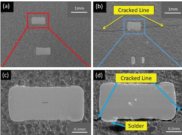
**Figure 5:** The SEM images of (a) top-down grinding of without RH treated sample (b) top-down grinding of RH treated sample (c) enlarged view of passive component of without RH treated sample and (d) enlarged view of passive component of RH treated sample
