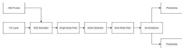
**Figure 1:** Tunable Multimode Fiber with Mode Division Multiplexing. Tunability of the filter is obtained by changing the incident angle of different beams at MMF.
