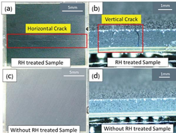
**Figure 4:** (a,b) Crack observed on RH treated sample and (c,d) no crack observed on non-RH treated sample
