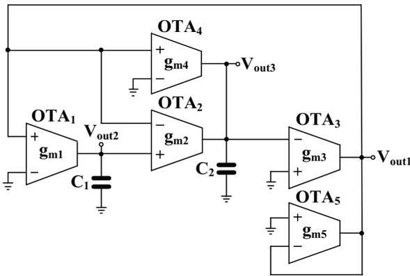
**Figure 3:** Three-phase quadrature oscillator modified from universal filter.
