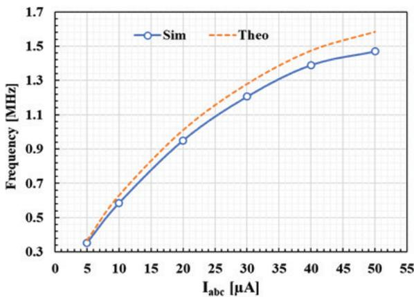
**Figure 16:** Simulated frequency of oscillation against biasing currents.
