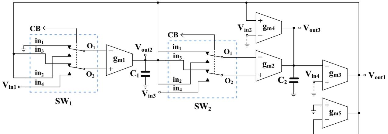
**Figure 4:** Proposed programmable filter and quadrature oscillator.
