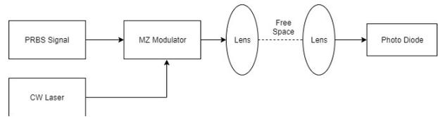
**Figure 8.** Basic Architecture of Free Space Optics
