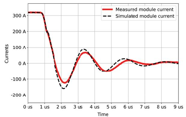
**Figure 11:** The  $I_{zdh} - I_{ce}$  current.
