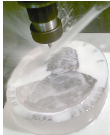
Fig. 18. Physical model manufactured by machining
