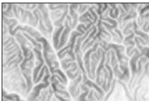
Figure 20: Surface slopes of DEM-100 with values between 0.00^\circ (lightest colour) and 18.15^\circ (darkest colour) for the Jeruzalem area.
