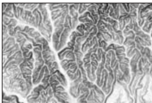
Figure 21: Surface slopes of DEM-25 with values between 0.00^\circ (lightest colour) and 32.80^\circ (darkest colour) for the Jeruzalem area.
