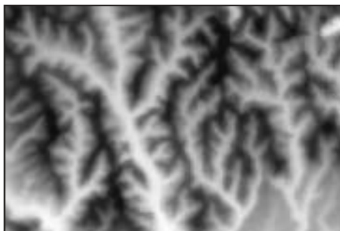
Figure 18: Surface heights of DEM-100 with values between 208 m (lightest colour) and 332 m (darkest colour) for the Jeruzalem area.
