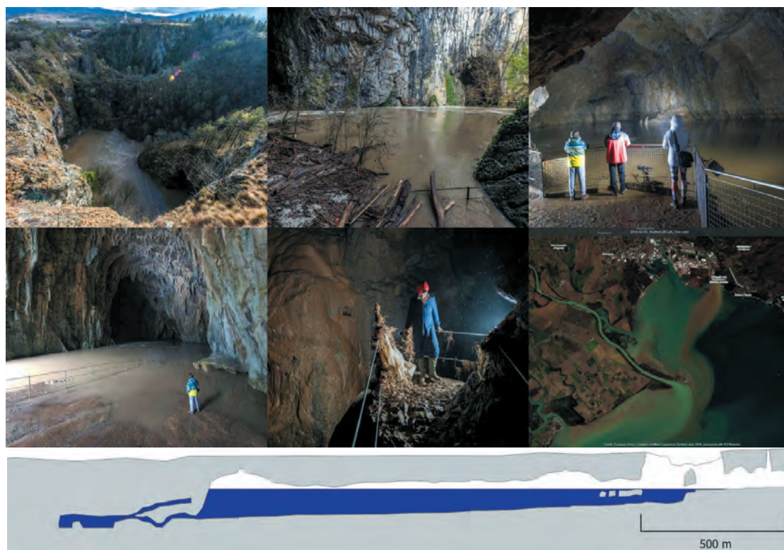
Figure 6: The water rose for over 90 m during flood in February 2019. The flood caused severe damage in infrastructure and deposited a thick layer of mud. Lower right: a satellite picture of Timavo springs region on February 5th (Photos: Borut Lozej, Škocjan Caves Regional Park, ESA Sentinel). Below: rough cross-sectional schematic view of water level during the 2019 flood.
