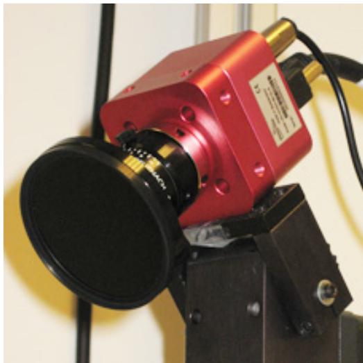
Fig. 1. 1 Megapixel camera with IR filter
