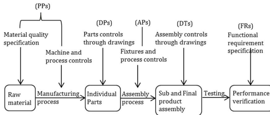
Fig. 4 Variables in discussion identified on production process
