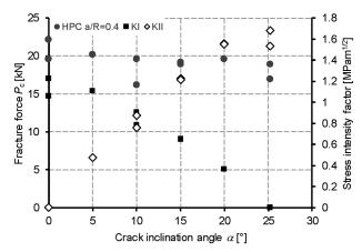
**Figure 2:** Fracture forces and values of SIFs for selected angles  $\alpha$  used for the BDCN measurement for a/R = 0.4
