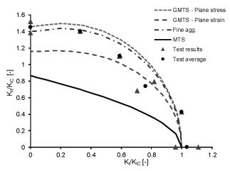
Figure 3: Mixed-mode I/II fracture-toughness diagram for the relative crack length a/R = 0.4
