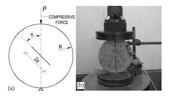
Figure 1: Brazilian disc with central notch: a) principle of testing and b) actual test setup
