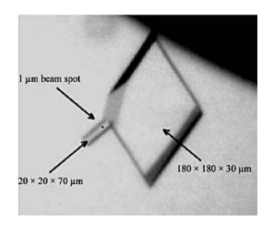
**Figure 5**: ESRF microfocus beam experiment; for the first time, a protein one-micron-beam-crystallography study has been performed ie with a focused synchrotron-radiation beam of 1  $\mu$ m using a goniometer with a sub-micrometre sphere of confusion. Thus the crystal structure of xylanase II has been determined with a flux density of about 3 × 10<sup>10</sup> photons s<sup>-1</sup>  $\mu$ m<sup>-2</sup> at the sample.<sup>27</sup> (reproduced with permission from ref. 27)
