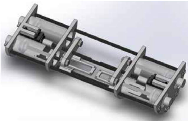
Figure 8 : 3D model of ballast tanks and submarine hull
