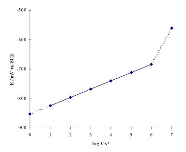
Figure 3. Response of the silver / silver sulphide electrode to the sulphide ion concentrations in 25% (v/v) SAOB
