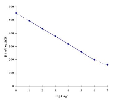
Figure 2. Response of the silver / silver sulphide electrode to the silver ion concentrations in 0.1 mol/L  $KNO_3$
