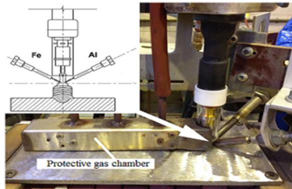
Fig. 3 Producing  $Fe_3Al$  using WAAM technology [16]
