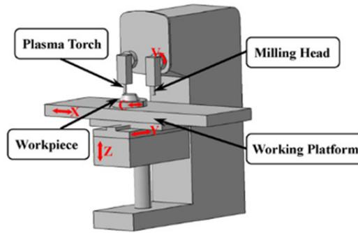
Fig. 7 CNC machine with welding torch and additional tool for milling [22]
