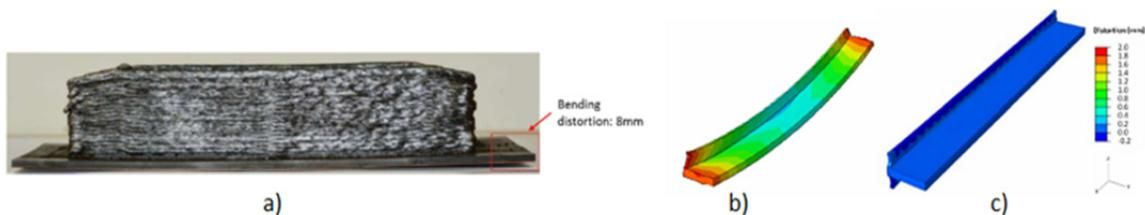
Fig. 5 Deformations (a, b) and solution through balanced building strategy (c) [5, 15]
