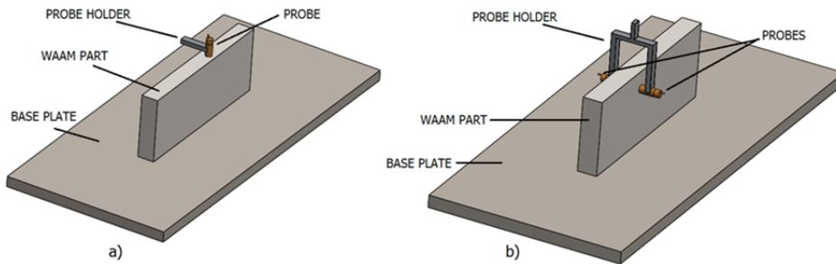
Fig. 8 Simplified preview of possible solutions for ultrasonic testing of WAAM parts
