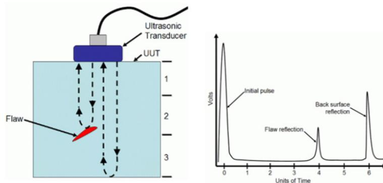
Fig. 6 Ultrasonic testing principle [26]
