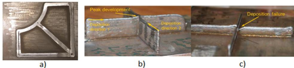
Fig. 4 Cavities (a), excessive camber (b) and sag (c) [1, 11]
