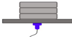
Fig. 9 Ultrasonic testing with probe on the bottom of the base plate
