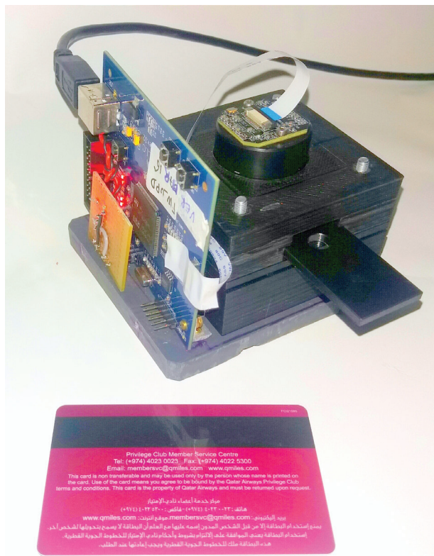
Figure 4: Hand held reader device, here shown with the case dismounted. A credit card in the forefront, is used for dimensional comparison purpose.
