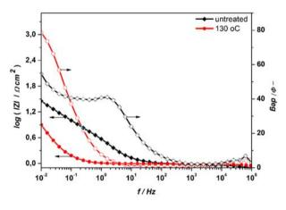
Figure 6. Bode plots of the thermally untreated  $\text{RuO}_2/\text{PVDF}$  sample (black curve) and one treated at 130 °C (red curve); binder/Ru-O<sub>2</sub> ratio = 0.1.
