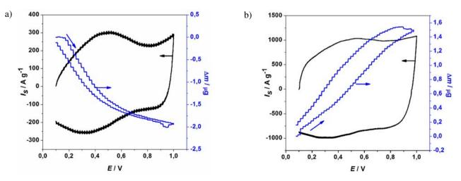
Figure 1. Simultaneous cyclic voltammograms and mass changes for the (a) hydrous, thermally untreated  $RuO_2$  and (b)  $RuO_2$  annealed at T = 130 °C. Scan rate: 0.2 V s<sup>-1</sup>. Electrolyte: 0.5 M H<sub>2</sub>SO<sub>4</sub>.
