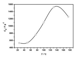
Figure 2. Dependence of specific capacitance of  $RuO_2$  on the temperature pre-treatment. Specific capacitances were calculated by the integration of the cyclic voltammograms recorded at 0.05 V.
