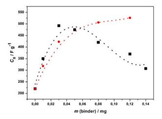
**Figure 4.** Characteristic dependence of the specific capacitance, Cs, on the mass of binder (squares – Nafion<sup>®</sup>, circles – PVDF) in the composite electrodes with  $m(RuO_2) = 0.1$  mg. Specific capacitances were calculated by the integration of the cyclic voltammograms recorded at 0.05 V.
