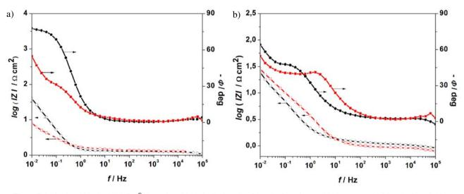
Figure 5. Bode plots of (a)  $\text{RuO}_2/\text{Nafion}^{\otimes}$  electrodes with binder/ $\text{RuO}_2$  ratio of 4, m( $\text{RuO}_2$ ) = 0.1 mg (black curve) and 0.86, m( $\text{RuO}_2$ ) = 0.46 mg (red curve); (b)  $\text{RuO}_2/\text{PVDF}$  electrodes with binder/ $\text{RuO}_2$  ratio of 0.25, m( $\text{RuO}_2$ ) = 0.1 mg (black curve) and 0.1, m( $\text{RuO}_2$ ) = 0.04 mg (red curve).
