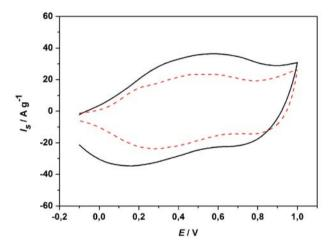
**Figure 3.** Cyclic voltammograms  $\text{RuO}_2/\text{Nafion}^{\otimes}$  (full line) and  $\text{Ru-O}_2/\text{PVDF}$  (dash line) electrodes with binder/ $\text{RuO}_2$  ratio of 0.25, m( $\text{RuO}_2 = 0.1 \text{ mg}$ ), examined in 0.5 M H<sub>2</sub>SO<sub>4</sub> electrolyte. Scan rate: 0.05 V s<sup>-1</sup>.
