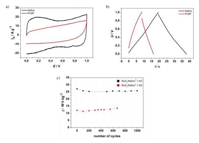
**Figure 7.** Electrochemical characterization of asymmetric  $\text{RuO}_2/\text{AC}$  capacitors. (a) Cyclic voltammograms of supercapacitors based on  $\text{RuO}_2/\text{Na-fion}^{\odot}$  (binder/ $\text{RuO}_2$  ratio = 0.25) and  $\text{RuO}_2/\text{PVDF}$  (binder/ $\text{RuO}_2$  ratio = 0.5) electrodes, m( $\text{RuO}_2$ ) = 0.1 mg; (b) galvanostatic charge/discharge curves for the two asammbled capacitors, (c) dependence of the specific energies during 1000 charge/discharge cycles.
