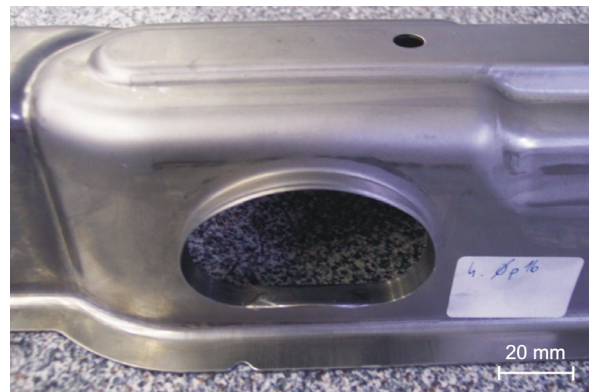
Fig. 9. Asymmetrical shape produced by BIHF, source: EMO-Orodjarna
