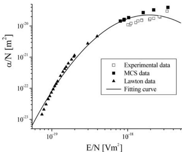
**Figure 3.** Comparison between experimental, Monte Carlo and Lawton data for ionization coefficients in oxygen<sup>18,19</sup>.
