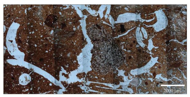
Fig. 5. Panoramic view of a pottery thin section of the kiln wall. The voids are the result of the burnedout organic material, straw. Photos taken under plain polarized light.
