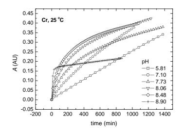
**Figure 4.** Formation of hydroxylated NPG derivatives followed by spectrophotometry at 431 nm, in Fenton-like reaction systems containing Cr(III) at 25 °C, the solution pH as indicated.
