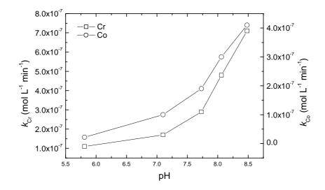
**Figure 5.** Rates of oxidising species production in Fenton-like reaction systems in the pH interval 5.5-9, at 25 °C for systems containing Co(II) and Cr(III), initially.
