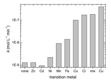
**Figure 7.** A comparison of rates of oxidising species production in Fenton-like reaction systems at pH 7 at 25 °C with transition metals as indicated.
