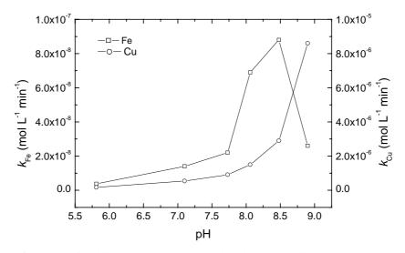
**Figure 1.** Rates of oxidising species production in Fenton-like reaction systems in the pH interval 5.5-9, at 25 °C for systems containing Fe(III) and Cu(II), initially.
