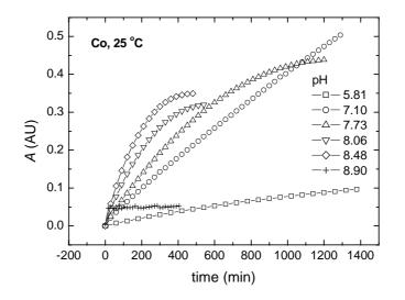
**Figure 3.** Formation of hydroxylated NPG derivatives followed by spectrophotometry at 431 nm, in Fenton-like reaction systems containing Co(II) at 25 °C, the solution pH as indicated.
