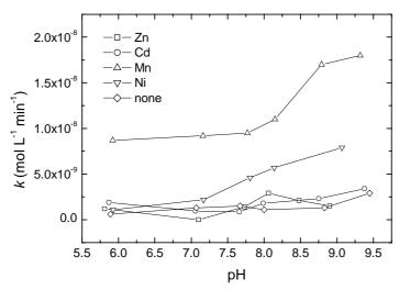
**Figure 6.** Rates of oxidising species production in Fenton-like reaction systems in the pH interval 5.5-9, at 25 °C with the addition of transition metals as indicated.
