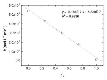
**Figure 2.** The effect of a mixture of Cu(II) and Fe(III) in Fenton-like reaction systems at pH 7, 25 °C on the rate of oxidising species production ( $\gamma_{Cu} + \gamma_{Fe} = 1$ , the summary concentration of transition metals 0.1 mmol L<sup>-1</sup>).
