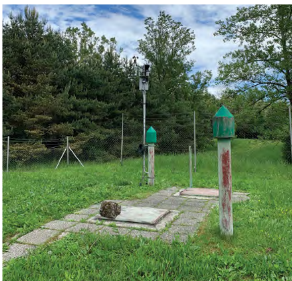
Figure 3: Measurement station Skorba V-2 for nitrate content in groundwater.
