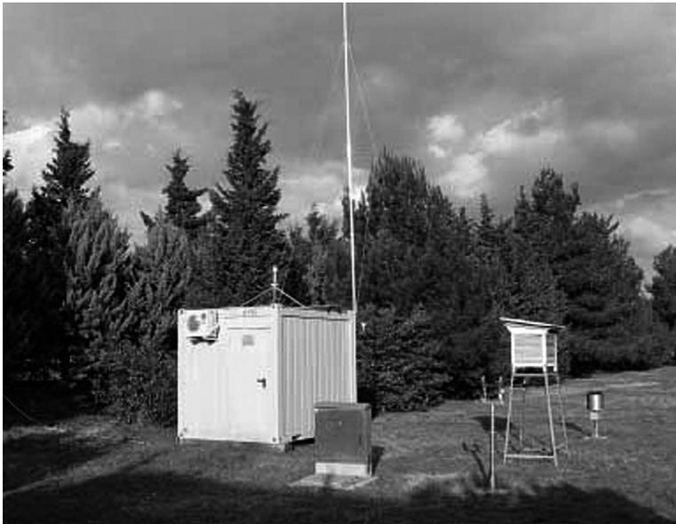
Figure 2: The continuous PM<sub>10</sub> particulate monitoring station (TEOM 1400A) in the Port of Koper
