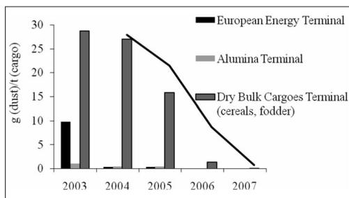
Figure 6: Annual emission levels of dust calculated in view of the total loaded cargo at different terminals
