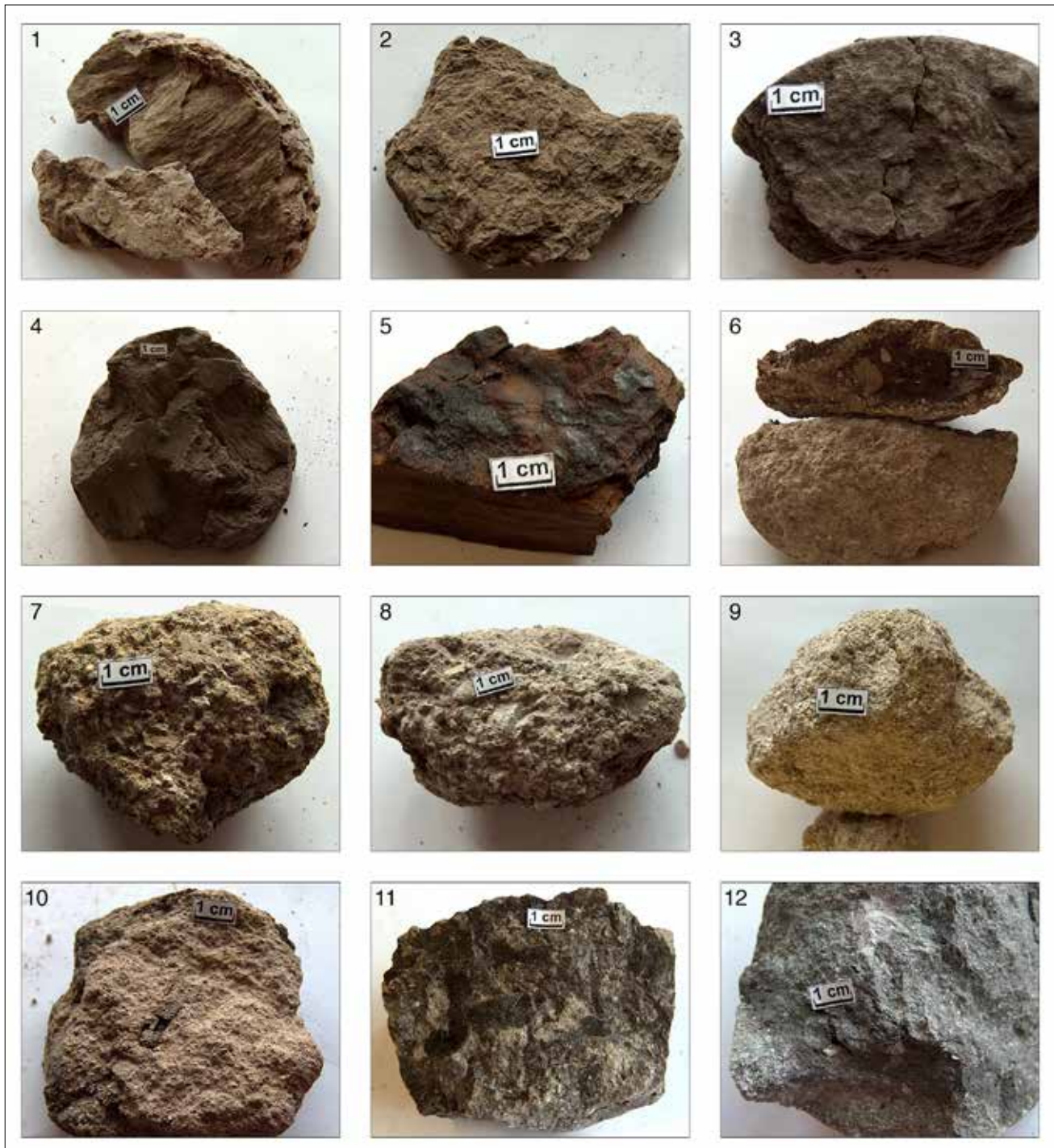
Fig. 5. Photographs of characteristic lithologic varieties: Photos 1–4 (samples 1c, 6, 9, 17): compact clayey silts; Photo 5 (sample 10a): siderite coated with geloxylite; Photo 6 (sample 2b): siderite concretion within sandstone; Photo 7 (sample 1a): gravelly sandstone; Photos 8, 9, 10 (samples 5a, 18 and 16): compact silty sands (photos 8 and 10) and a gravelly sand (photo 9); Photos 11 and 12 (samples 19b and 20): lithified slightly gravelly calcite-cemented quartz sandstones.
