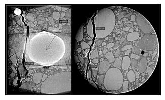
**Figure 1:** 2D slice in the *XY* direction of the steel bar embedded in the concrete (left image). A layer of the secondary corrosion products is visible on the surface of the embedded bar (the bright layer) as well as on the surface of the newly formed crack (left and right image). The cracks in the concrete cover were formed due to the increased volume of the secondary corrosion products.
