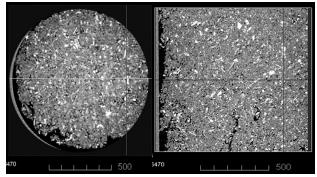
**Figure 5:** Horizontal slice (left) and a vertical slice in the *XZ* direction (right) of the humid-soil specimen in a glass capillary, partly visible on the left image. Different inorganic (brighter) and organic (darker) components are visible in the figure, as well as the cracks and air voids. A snapshot of a 3D representation of the soil structure is given in **Figure 6**.
