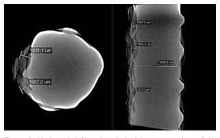
Figure 2: Horizontal (left) and vertical (right) cross-sections of the corroded steel bar. Approximately two millimeters of the bar was corroded due to the exposure.
