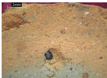
6. Renče clay, fired at 800°C, Sample 7. 8x magnification Leica Stereomicroscope EZ4.
