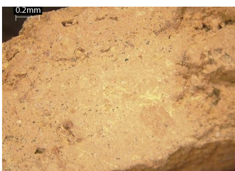
3. A thin section of a vessel fired in a kiln at 670°C. 8x magnification Leica Stereomicroscope EZ4.
