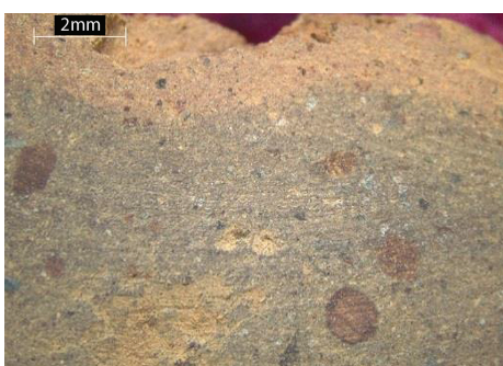
5. Renče clay, fired at 600°C, Sample 6. 8x magnification Leica Stereomicroscope EZ4.
