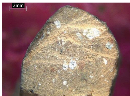
8. Renče clay with admixed calcite, Sample 12. 8x magnification Leica Stereomicroscope EZ4.
