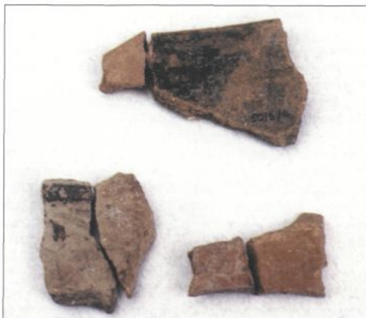
Fig. 6. Refiring of sherds from Promachon-Topolnitsa decorated with an organic coating. In the clear coloured chips of two of these sherds the organic material disappeared after refiring at 450°C, for 30 minutes. The pink-red slip of the third sherd was not affected by the firing.
