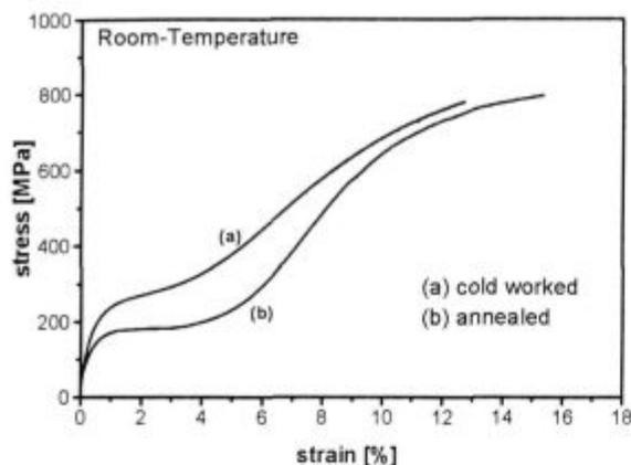
Figure 1: Stress strain curves of the martensitic modification
