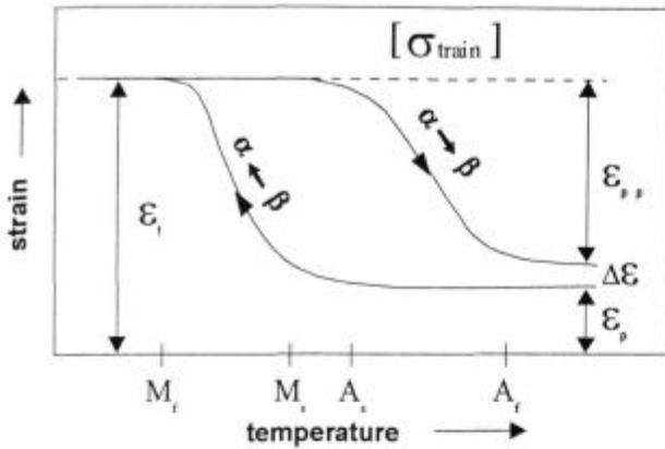
Figure 3: Schematic illustration of a training cycle indicating the labelling of the different strains:  $\epsilon_t$ : total strain,  $\epsilon_{pp}$ : pseudoplastic strain,  $\epsilon_p$ : irreversible strain
