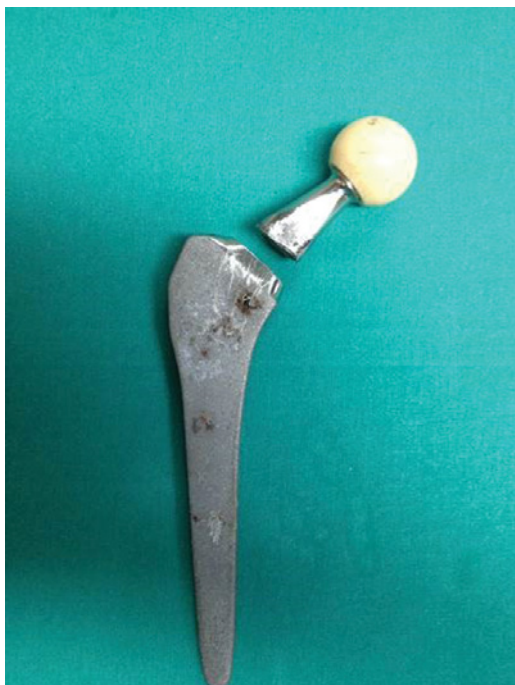
Figure 1: A Profemur Z implant femoral stem after explantation at the revision total hip arthroplasty. The fractured modular neck with a ceramic femoral head still attached.
