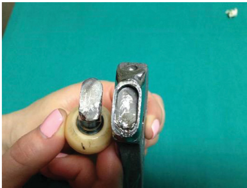
Figure 2: A fractured modular femoral neck. The distal part is still in the female part of the Morse taper of the femoral stem.
