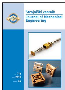
**Cover:** Exploded view and partly assembled prototype of a new hydropowered surgical drill. The prototype is on scale and based on an external gear motor, where one gear is extended with a drill bit. Experiments were performed at the Laboratory of Material Sciences, Faculty of Mechanical Maritime and Materials Engineering, Delft University of Technology, The Netherlands and the Laboratory of Austrian Center for Medical Innovation and Technology, Wiener Neustadt, Austria.
