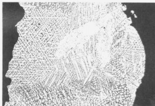
Figure 2. Dendritic microstructure in particles > 1400 \mu\text{m} .
