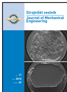
Cover: SEM image of failure types on spot welding samples after tensile-shear test for different welding distance of adjacent spots to investigate shunting effect on AA2219 sheet
