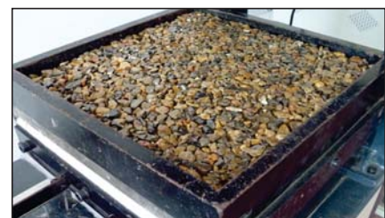
Figure 4. PUR mixed crushed stones.
