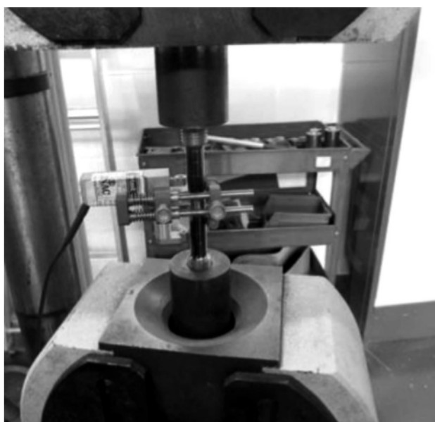
Figure 1: Tensile testing machine and extensometer
