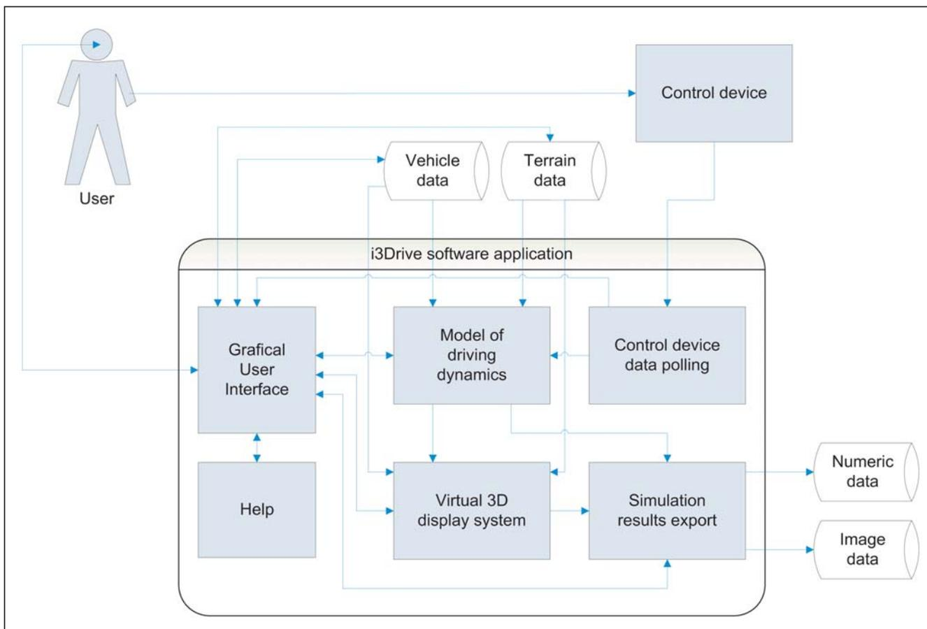
Figure 3. *i3Drive application scheme*
