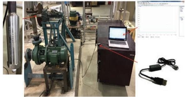
Fig. 3. Data acquisition and processing system for pressure fluctuations
