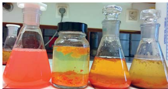
Slika 9: Od leve proti desni: izhodiščna odpadna voda suspenzije tiskarske barve, odpadne vode, čiščene z mandarininimi olupki, s pomarančnimi olupki in z avokadovimi olupki v koncentraciji 12,5 g/l Figure 9: From left to right; initial printing ink wastewater, wastewaters treated with mandarin peels, with orange peels and with avocado peels in concentration of 12.5 g/l
