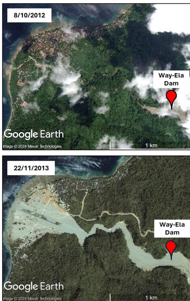
*Figure 2: Way-Ela Dam before (October 2012) and after (November 2013) the dam-break (Google Earth.)*
